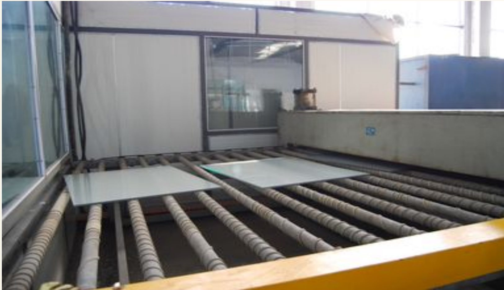
8- Glass into Flat Pressing Machine
