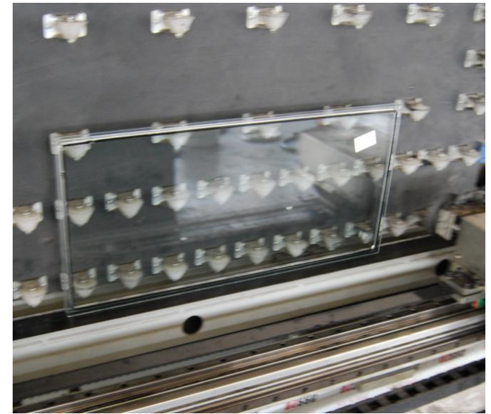
6. The glass glazed before sealed
